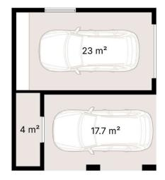
This dual-section garage offers a unique design, featuring a 17.7m² carport for one vehicle and an additional 23m² enclosed garage for another car or a spacious storage or workspace. The design includes a dedicated 4m² storage room, ideal for tools or garden equipment, providing added flexibility and functionality.
